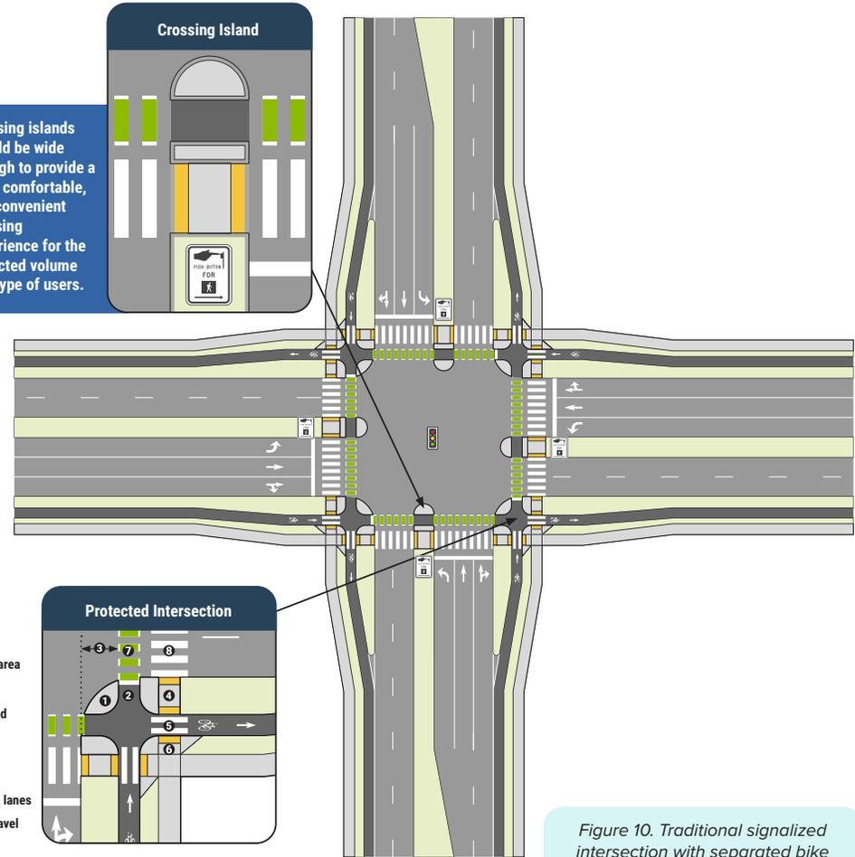
Figure 10. Traditional signalized intersection with separated bike lanes. Source: FHWA.
