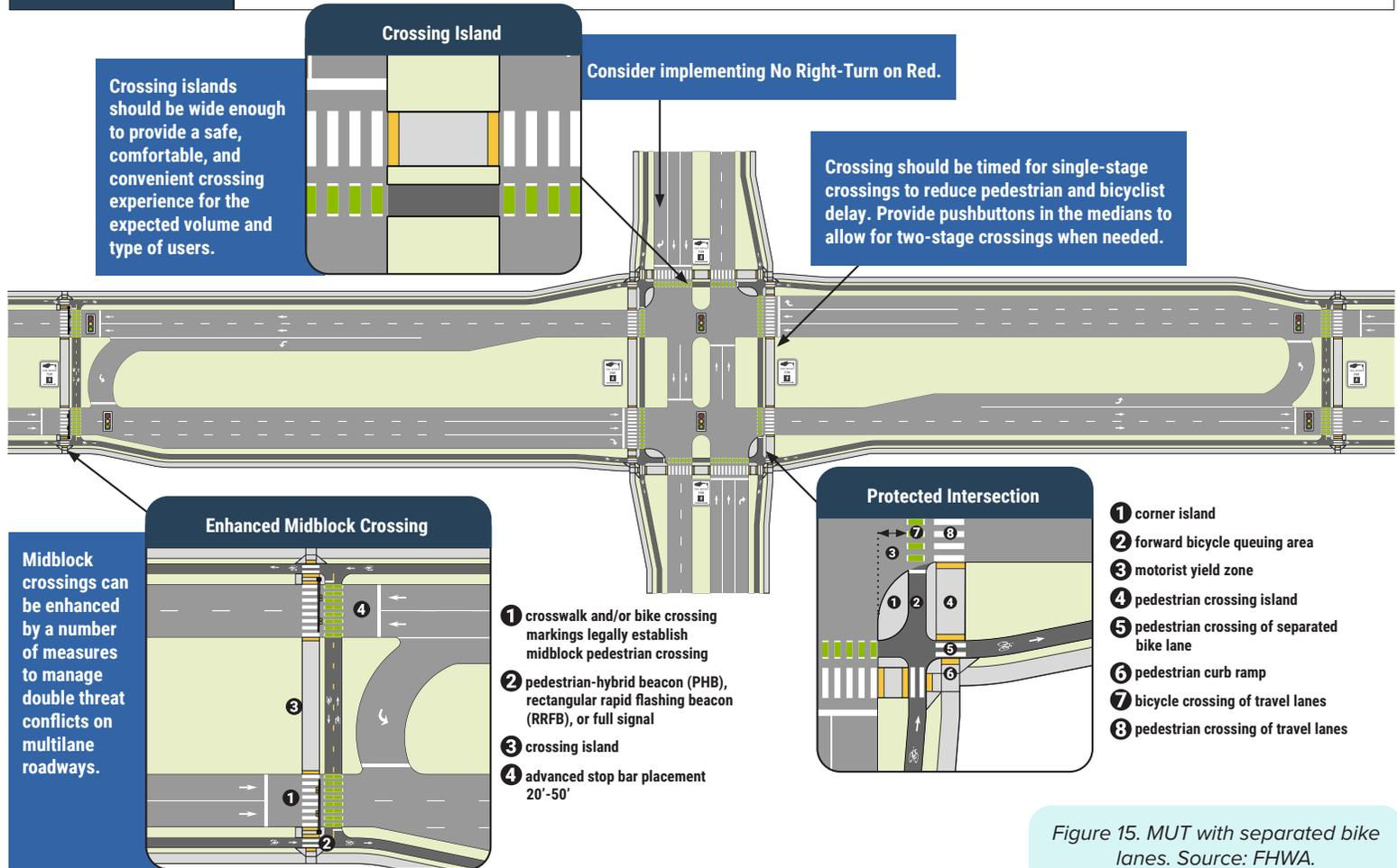
Figure 15. MUT with separated bike lanes. Source: FHWA.
