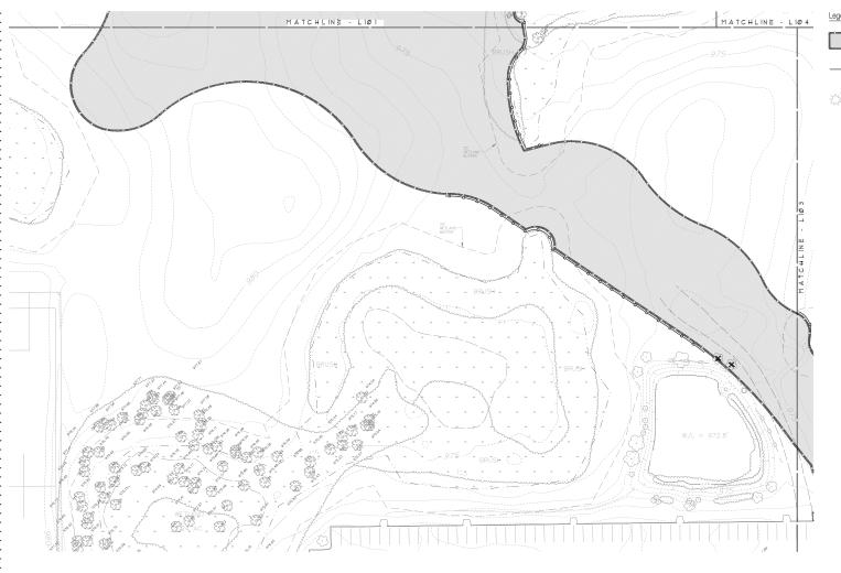
LIMIT OF BORK AREA BITH SILT FINCE -SEE CIVIL DOCUMENTS FOR DETAIL UETLAND / UDODLAND PROTECTION PENCING UITH SILT PENCE (SEE DETAIL ON SHEET LIGH)
