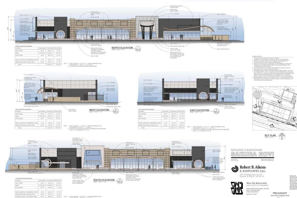
NOTE : 1. TOTAL FACADE = 5,456 5.F. - GLASS STOREFRONT AND DOOR AREA OF 1,354 5.F. = 4,102 5.F. 2. NO SECTION 9 FACADE WAVEFES ARE REQUIRED.
