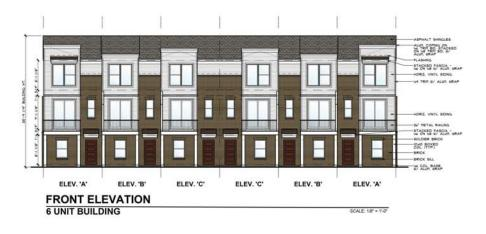
FRONT ELEVATION ALLOWABLE PROPOSED PERCENTAGE MATERIAL 1,018 SF 38.5% BRICK 100% SIDING 0% 422 SF 23.5% SHINGLES 25% 449 SF 17% TRIM 15% 551 SF 206 TOTAL 2,440 SF 100%
